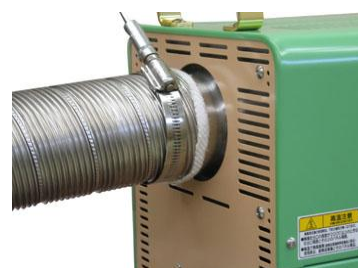
Execution example of the glass tape for air leakage prevention
